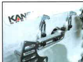
Closed window for Needle thread take up to avoid oil leak
