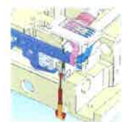
Oil return device in feed dog shield cover
